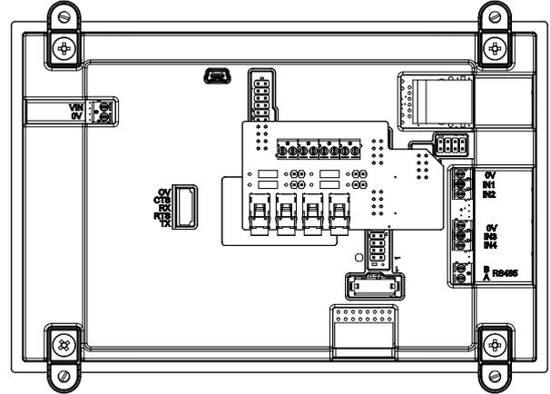
The diagram (above-right) indicates the pins on the SGD 70-A that the S70-TP should be connected to.
