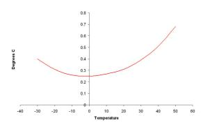
The reading resolution and reading accuracy of this unit are the same
