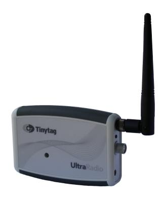
Tinytag Ultra Radio data loggers are a range of wireless data loggers products designed for indoor use. The loggers are used as part of a Tinytag Radio system that forms a robust data network that allows a user to see the conditions within an application from their own desk, across a LAN or the Internet.
