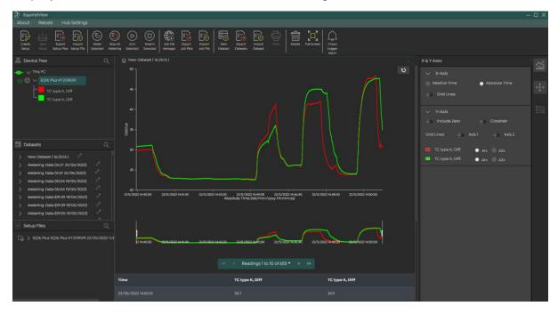
Options for changing the graph display and formatting the data are available through the menu tabs on the right side of the display. Here you can edit the graph type, change the title of the graph, alter the x and y axis and add threshold limit values:
