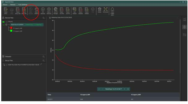
Meter mode allows you to view data from all measurement channels at a frequency of 1 reading per second in real time.
