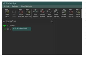
The Logger is now connected. The software will detect what type of logger it is and display the type and serial number. For a full list of data logger products this software will support refer to the specification table.
