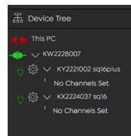
The Plug icon will change to Connected **P** and the loggers will appear in the Device Tree with the logger serial number followed by the logger model type sq16 or sq16plus.In this example KY2221002 sq16plus.
