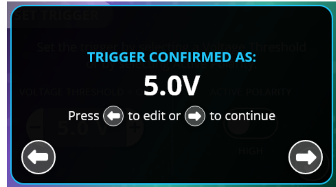
Fig.4 Trigger Confirmation Screen (Voltage Threshold)
