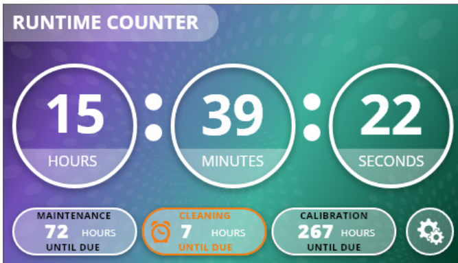
Fig.14 80% Amber Alarm Alert
