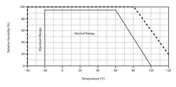
Long term exposure (more than 60 hours) to conditions outside the normal range, shown above, may result in a temporary drift of up to +3% RH. Once within the normal range again it will return to the calibrated state.
