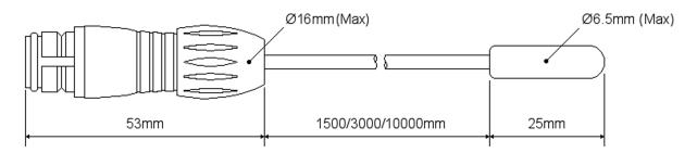
Typical Applications Composting Cable lengths
