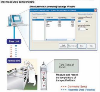
To further help meet our customers need, we offer the RTR-61 Communication DLL. By using our RTR-61 DLL, you can create software on your own for your own situation and purposes. The following are the examples of the DLL functions: Control of Base Unit Functions via Computer, Remote Measurement Command, Downloading Data, Sending / Getting Tables. For details please contact your local T&D dealer.
