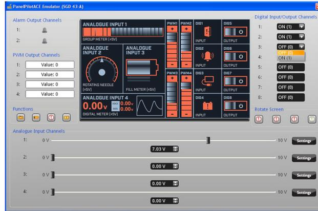
Design Studio includes a 'Preview in Emulator' function which emulates the hardware inputs/outputs allowing you to test projects prior to upload. Projects are uploaded to the PanelPilotACE display via USB.
