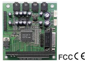
The kernel of PCM-3201 is the ALS120 chip that are industry standard music synthesizers found in most personal computer audio boards. The PCM-3201 brings cost-effective Wave Table synthesis capability to the PC/104 form factor. The ALS120 single chip audio solution integrates audio CODEC and DOS games compatibility, plus, minimizes support and installation issues.
