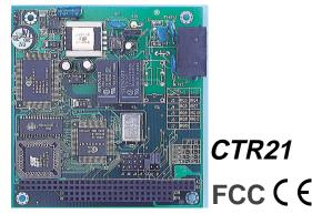
The PCM-3601 uses Rockwell®DSP, which meets standard 56K bps maximum data transmission speed without additional CPU loading. It also supports the G3 fax standard of 14.4 K fax transmission rate and full duplex functionality. The PC/104 form factor makes it a great fit for space-limited and harsh environment applications.
