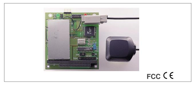
The PCM-3291 GPS module is designed with sophisticated satellite technology to locate and track any location in the world, in real-time. Using a Rockwell®12-channel GPS engine that provides differential input for use of DGPS to assure pinpoint accuracy, the PCM-3291 offers a wide range of GPS functions such as position, navigation, satellite and timing information for use in embedded-PC navigation systems.
