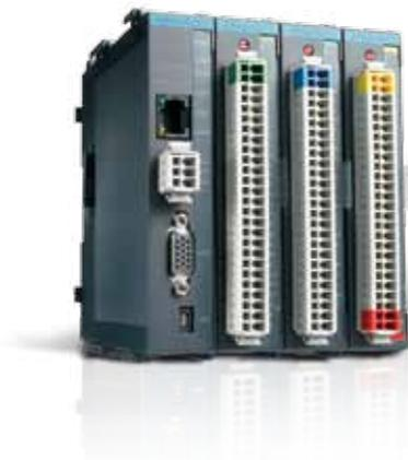
APAX-5520/5620 series controllers offer a compact size without fans. These controllers have no rotating parts, helping further increase system reliability. APAX-5520/5620 features a VGA interface, enabling local displays, and its RS-485 and LAN ports offer communication ability with Modbus protocol. Internal CF slot and battery backup RAM can be used for data storage. These features make APAX-5520/5620 as compact and robust as a PLC, but with enhanced displays, connectivity, and storage.
