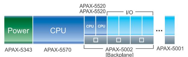
Note: The APAX-5570 can be upgraded to APAX-5571, APAX-6572, etc.
