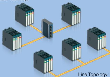
All APAX I/O modules are inserted on the backplane. Through the expansion port and Ethernet cable, different backplanes can be connected. This decentralized architecture retains high-speed data transfers, so the distributed I/O modules provide real-time performance. Almost any topology, such as line, tree or star, can be easily established. The hot swap capability is also available for remote expansion I/O modules.
