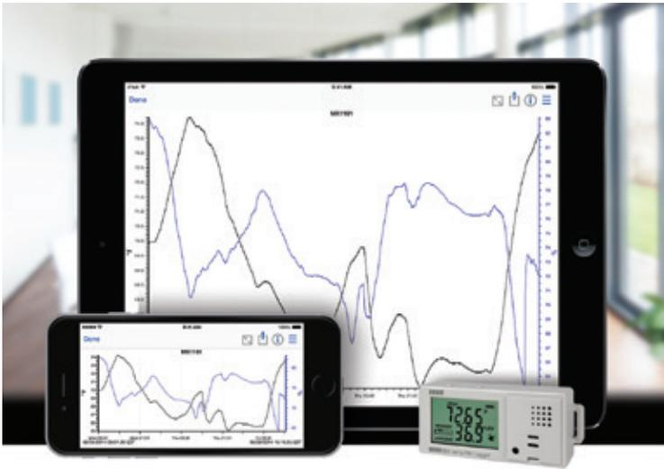
HOBOMobile™ is designed to enable communication between a Bluetooth® Smart mobile phone or tablet and the HOBO MX series data loggers. You can configure and start the data logger, download the recorded data, and store and analyze the data. The HOBOMobile app is a free download. See pages 1-2 for more details.
