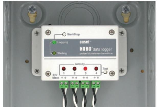
**Supported Measurements:** Pulse Signals, Event, Runtime, State, AC Current, AC Voltage, Amp Hour, Kilowatt Hours, Kilowatts, Motor On/Off, Power Factor, Volt-Amps, Watt Hours, Watts, Volt-Amp Reactive, Volt-Amp Reactive Hour (sensors sold separately)
