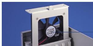
A 49-CFM cooling fan for easy-replacement and maintenance
