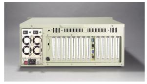
Rear panel of backplance version with redundant power supply
