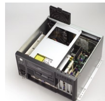
Solid disk drive housing & easy-to-maintain fan filter
