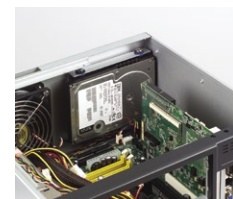
Shock-resistant drive bay designed to hold an internal 3.5" HDD
