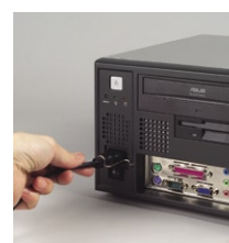
Plug ring-lock securely fastens the power cord
