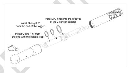
3. Install two O-rings onto the MX801 logger (see above). The O-rings serve to stabilize and center each part of the assembly.
