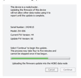
When the firmware is saved to the device, the LED will flash red on the receiver and green on a data node. A message appears at the end when the update is successfully completed.
