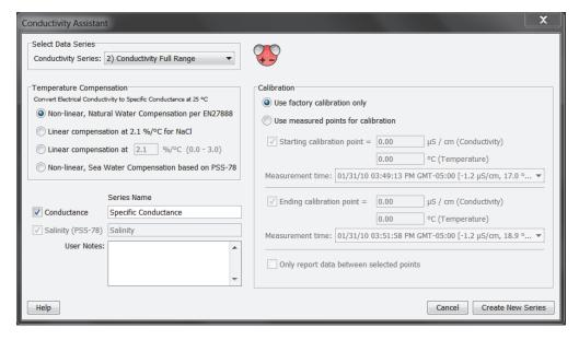
• For the U24-002-C logger, select either Conductivity Low Range when the data is always less than 10,000  $\mu$ S/cm or select Conductivity High Range (default) when the data goes above 10,000  $\mu$ S/cm as shown below.
