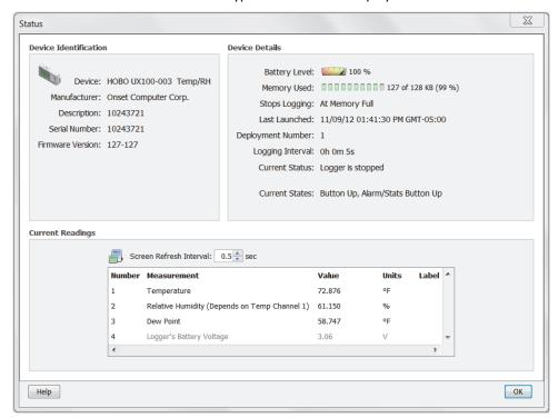
**Important:** Battery power is drained more rapidly while checking status. Keep this in mind when frequently checking status during a deployment. You can significantly reduce the demand on the battery by adjusting the Screen Refresh Interval to five seconds or higher (not available on all loggers).
