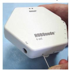
To later reactivate the data node, select Form Network from HOBOnode Manager and briefly depress the Activate button on the node.
