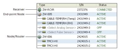
For another way to see whether the device is a data node only or a data node/router, double-click the device to open the Configure Node dialog. Check the Device Type for the device part number and description. In the example below, the device is operating as a both a data node and a router so the Device Type is listed as "ZW-006 (Node/Router)." If this device was powered by batteries only, then it would be operating as a data node and not a router, and listed as "ZW-006 (Node)."
