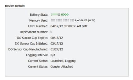
In the Device Details pane, three key DO sensor cap dates are displayed:
