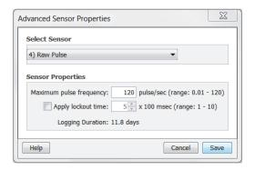
3. Click the "Apply lockout time" checkbox if you wish to specify a time period when pulses will be ignored. Select the lockout time value from 1 to 10. On sensors with both pulse frequency and lockout time settings, lockout time will affect the maximum pulse frequency: the higher the lockout time, the lower the maximum pulse frequency will be.
