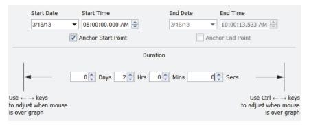
As another example, to set a range of 1 day ending at 10:00 PM on 3/18/13, set the End Date to 3/18/13 and the End Time to 10:00:00.000 PM. Select the Anchor End Point checkbox and set the Duration to 1 day.
