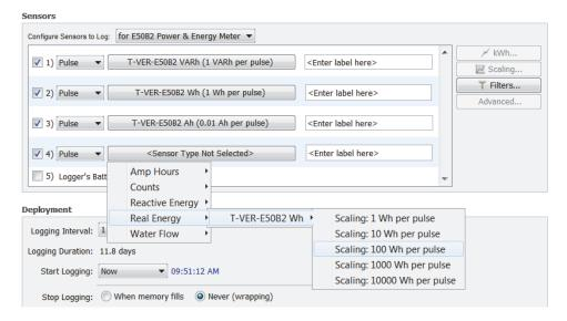
3. Select any other Launch settings as desired and then click Start to launch the logger with the Onset Power Meter settings (note that the Start button name changes depending on when you chose to begin logging).
