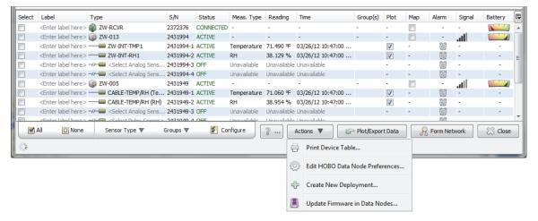
Follow these steps if you are directed by Onset Computer to upgrade the firmware in multiple data nodes. To update the firmware in the receiver or in a single data node at a time, see Updating Firmware for a Receiver or Single Data Node.
