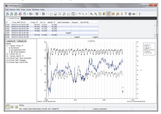
This example shows a file that has been opened and plotted. There are three components to a plotted datafile: the Points Table, the Details Pane, and the Plot.
