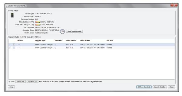
4. Click the Offload Checked button when you are ready to begin offloading the files from the shuttle. Once offloading begins, the Offload Checked button will change to Cancel Offload. When offloading is complete, the Files on Shuttle panel in the Shuttle Management window will change to a Files Offloaded From Shuttle panel.
