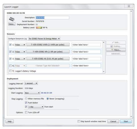
When these settings are selected, the logger will record the default values from the Onset Power Meter. This means that when you read out the logger, the first three data channels will record the following by default:
