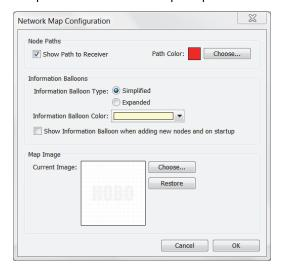
In the Node Paths pane, select the Show Path to Receiver checkbox Paths to show or hide connection paths between nodes. To change the path color, click the Choose button. Select a new color from the Swatches tab, or enter HSB or RGB values and click OK.
