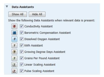
When you read out a logger or open a datafile, all compatible Data Assistants are listed in the Plot Setup window by default. Deselect the checkboxes for any assistants that you do not want to display in the Plot Setup window. Or, click Show All to display all compatible assistants in the Plot Setup window or Hide All to display none of them.
