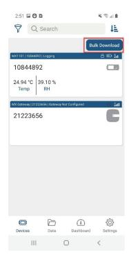
The screen changes to Bulk Download mode. This changes the way the screen behaves when you tap on a logger tile. Tap on a tile to select it for Bulk Download. You can select up to 20 loggers. Text at the bottom of the page updates to indicate how many loggers are selected.
