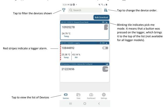
Loggers in alarm state are listed first. If you've pressed a button on a logger to wake it up (not available on all logger models), that logger is at the top of the list. By default, all other loggers are listed in ascending order by discovery time.
