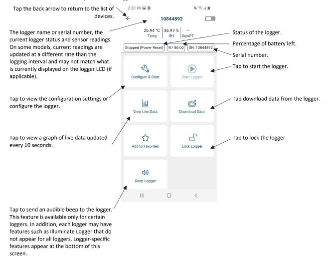
**Note for MX2001 loggers:** When the logger is stopped, the water level reading does not reflect any reference water level and water density values you have entered (it reverts to a reference water level of zero and a water density of "Fresh Water adjusted for Temperature"). Once logging begins, the readings are then based on the reference water level and water density you entered.
