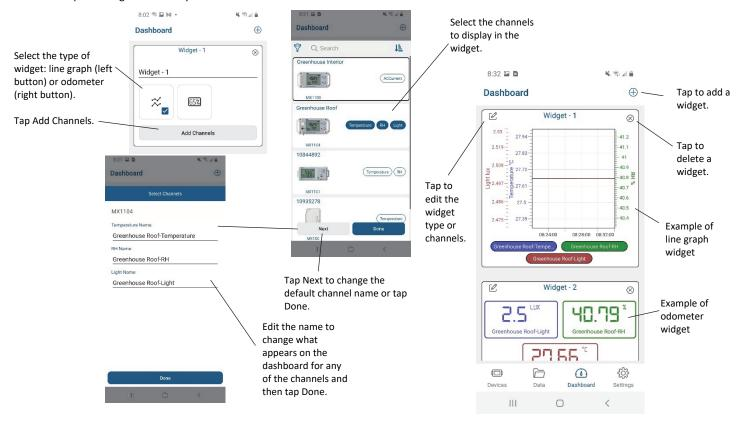
Measurements are updated every second when the logger is within range. Note that measurements displayed on the dashboard may differ from logged data points, which are recorded at the logging interval selected when configuring the logger. When a logger is out of range, the graph widget will not display any measurements and the odometer widget will display the most recent measurement from when the logger last communicated with the phone, tablet, or computer.
