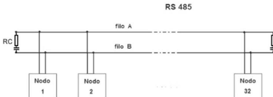
By way of example, the value of the capacitor will have the following values depending on the length of the line: 10 nF (150 m) - 22nF (300 m) - 47 nF (600 m) - 100 nF (1000 m).
