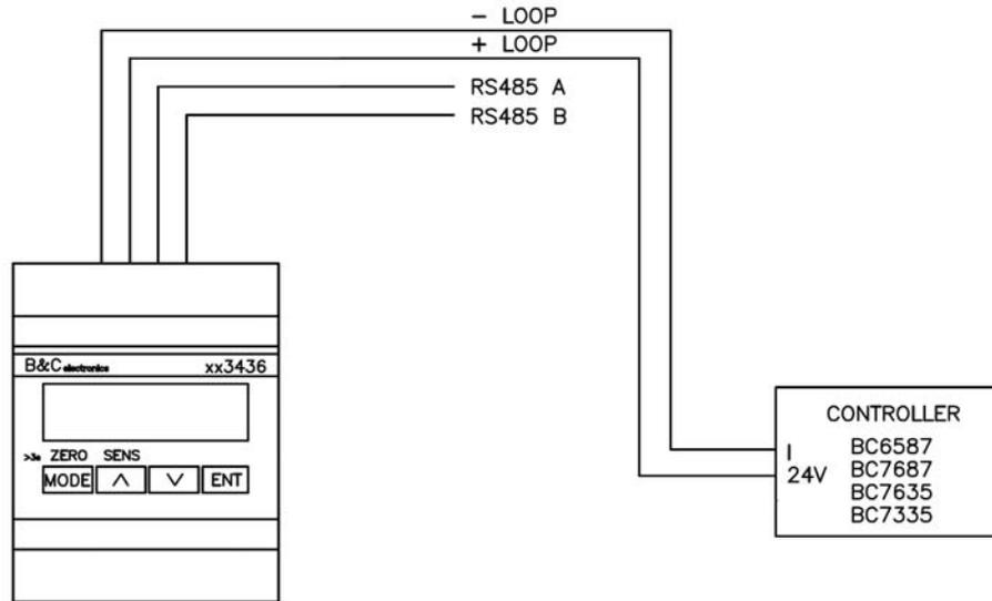
*Connection to B&C Electronics' instruments*
