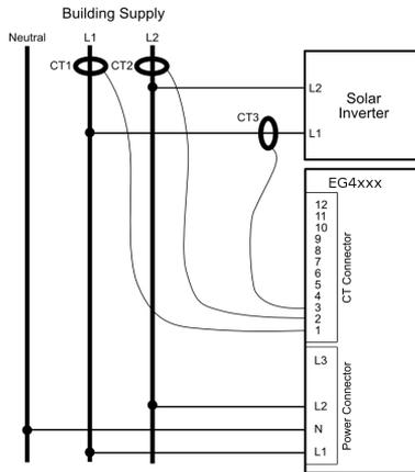
Figure 8: Wiring Diagram for a Typical Split-Phase Installation
