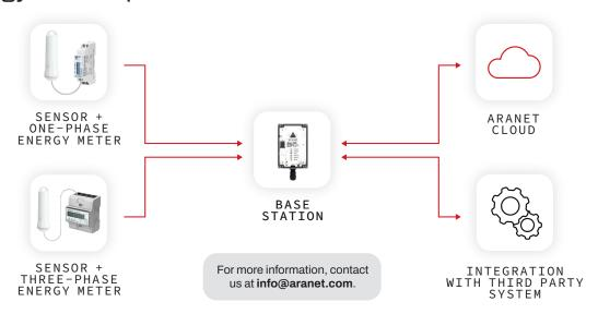
An <u>Aranet Base Station</u> combined with a <u>Dry Contact Pulse Counter</u> sensor and a <u>one-phase</u> or <u>three-phase</u> energy meter allows easy tracking for the consumption of electric energy remotely and from one place.
