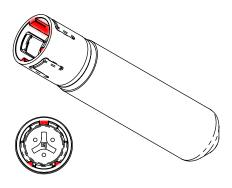
Reinstalling the probe: Before installation, ensure that the highlighted indentations between the probe and socket are aligned.
