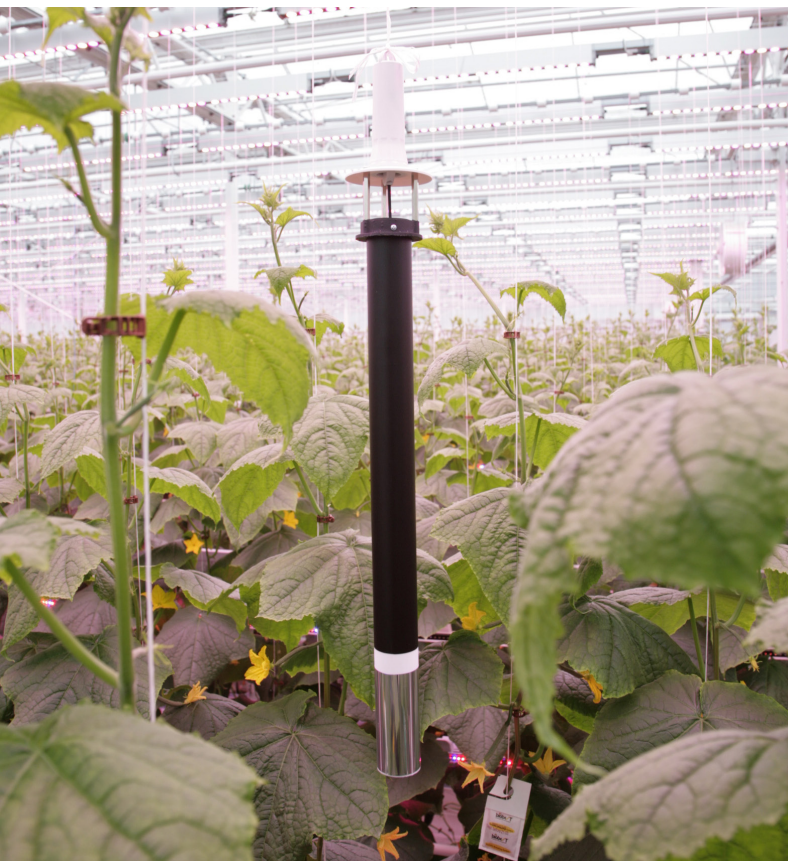
Aranet T/RH sensor with Convection Radiation Shield
