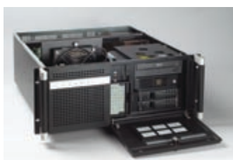
Easy-to-maintain system fan & reusable filter design
