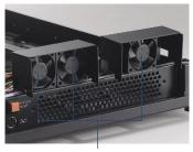
Three filtered 10-CFM cooling fans are on front-end
