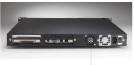
One 10-CFM cooling fan is on rear-end
