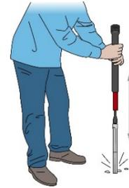
5. Once the pilot rod reaches the desired depth, extract the pilot rod by using the slide hammer in reverse, lifting it rapidly to hammer upwards.
