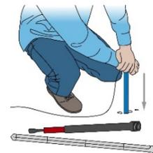
8. Pack the soil around the top of the sensor to prevent water from entering the hole. The sensor should be completely covered with soil and only the sensor cable visible.
