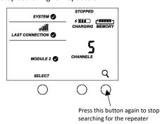
When you are finished adding repeaters and wireless sensors to the network, the total channel count for the module on the station will represent the measurement channels from all motes plus a battery channel for each mote (including repeaters) in the network.
